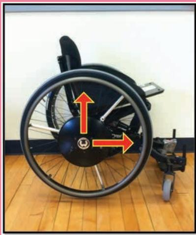
**FIGURE 2** REAR AXLE POSITION (RAP) - Moving RAP up and forward relative to shoulder can improve propulsion biomechanics
