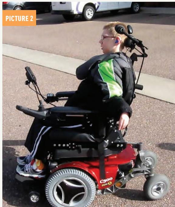
Driving with the head array in a demo chair
